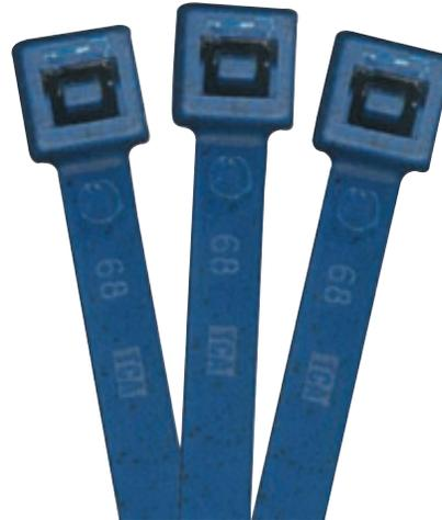
**Product Description:** Detectapro's metal detectable cable ties feature a food safe metal additive, dispersed evenly and completely throughout the entire polyamide 6.6 body of the cable tie. These cable ties have an operating temperature of -40°F to 185°F, and can be used as part of a HACCP process or BRC procedures. These cable ties come in a standard colour of blue, making them visually detectable, further reducing food contamination risks.
